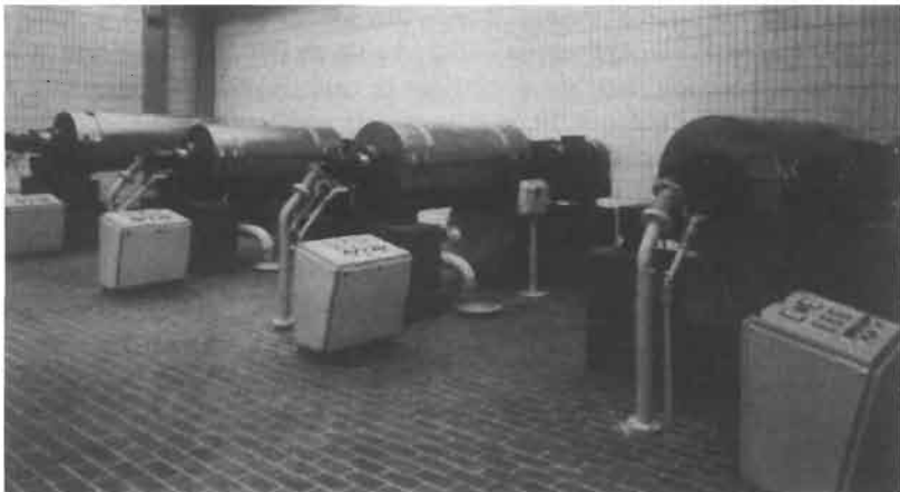
Figure 10-15. Solid bowl centrifuges. (Photo courtesy of Ingersoll Rand and I. Krüger.)
