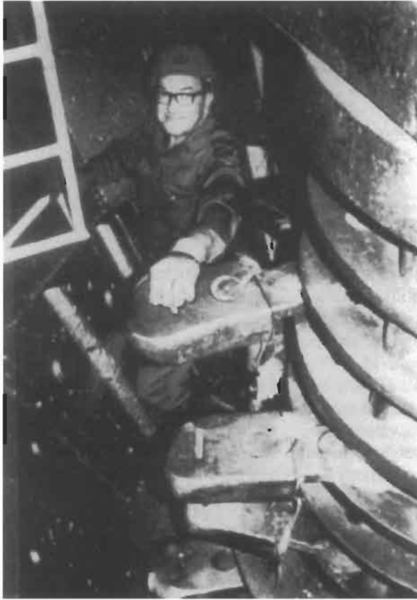
Figure 14-3. Inside a vertical hammermill. The hammers have been worn down by the shredding process. (Photo courtesy of W. A. Worrell.)
